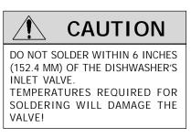
\* Water inlet valve located at the bottom left front of the dishwasher.
